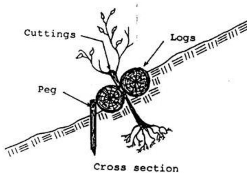
Figure 85. Ground tie with sprouting brushwood (Source: Manual of Reforestation and Erosion Control, Agpaoa *et al.*, 1975)
