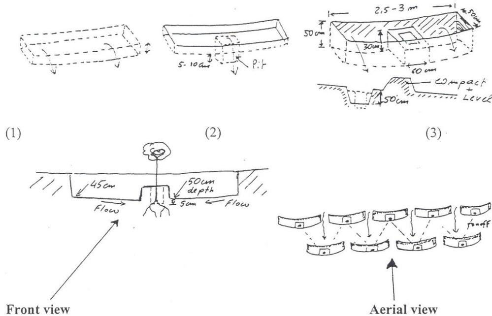
Figure 57. Design of water collection trenches
