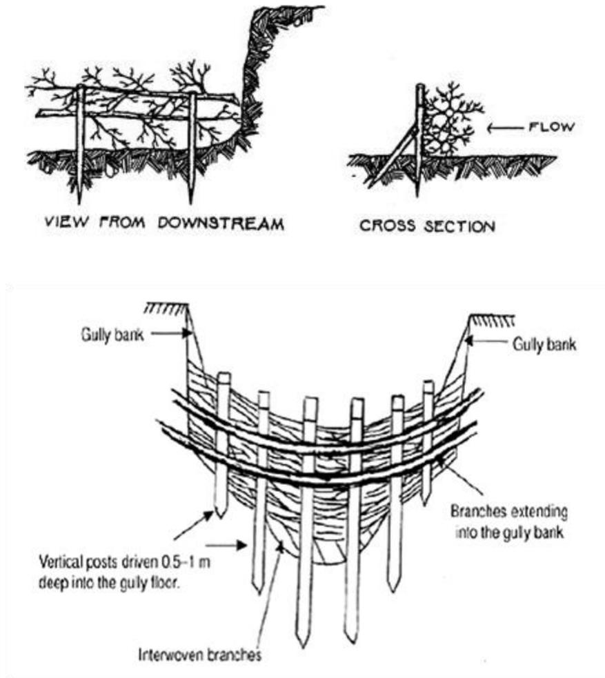
Figure 82. Brushwood checkdams (Source: Manual of Reforestation and Erosion Control, Agpaoa *et al.*, 1975)
