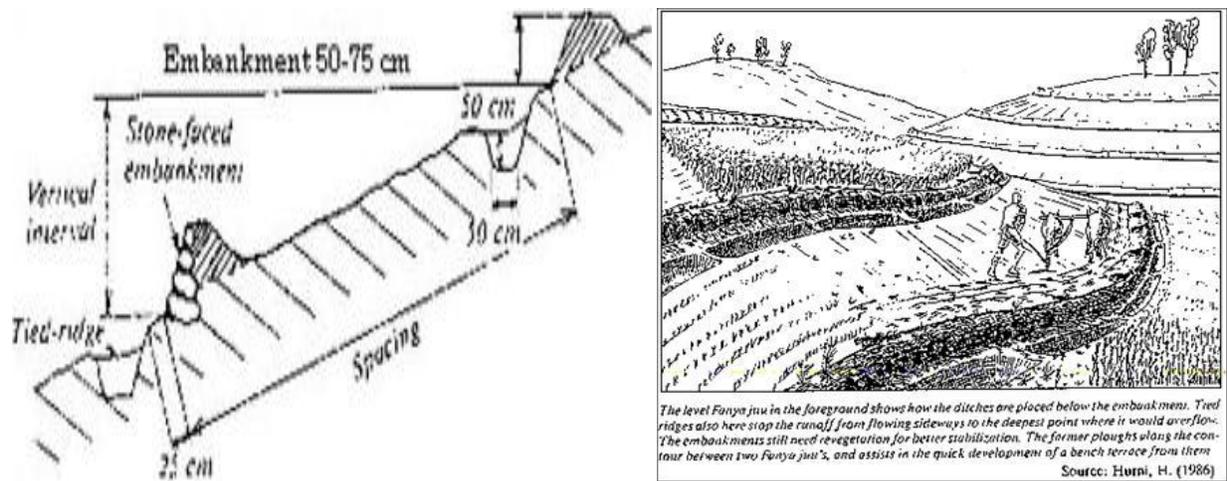
Figure 53. Design of Level Fanya juu, schematics and terminologies
