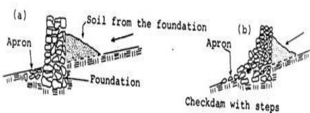
Figure 79. Dry stone checkdams (Source: Manual of Reforestation and Erosion Control, Agpaoa *et al.*, 1975)
