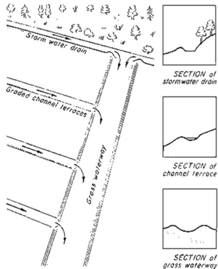
Figure 68. Grass water way and the input system sections
