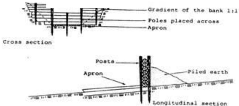
Figure 83. Pole or log checkdam (Source: Manual of Reforestation and Erosion Control, Agpaoa *et al.*,1975)
