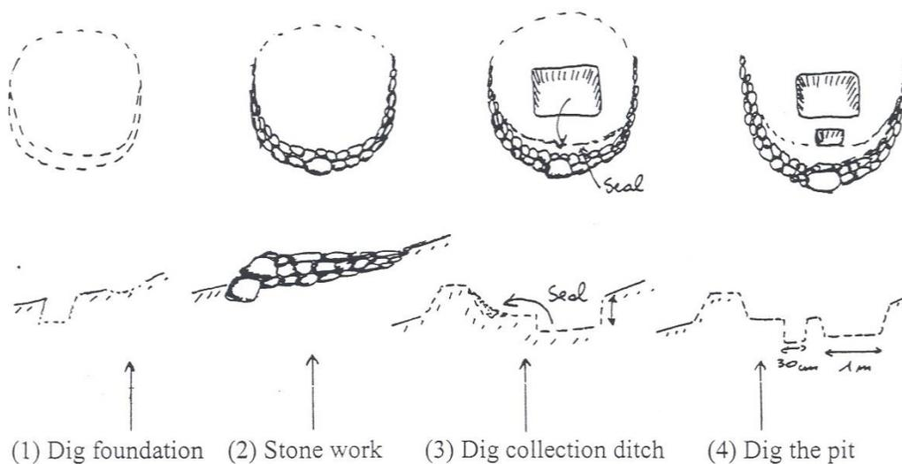
Figure 62. Construction steps of eyebrow basins
