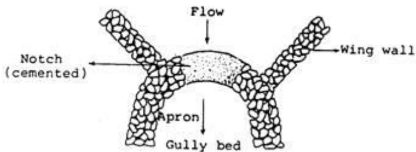
Figure 76. Gully head stabilisation by a solid structure with wing walls (view from above) (Source: Manual of Reforestation and Erosion Control, Agpaoa et al., 1975)
