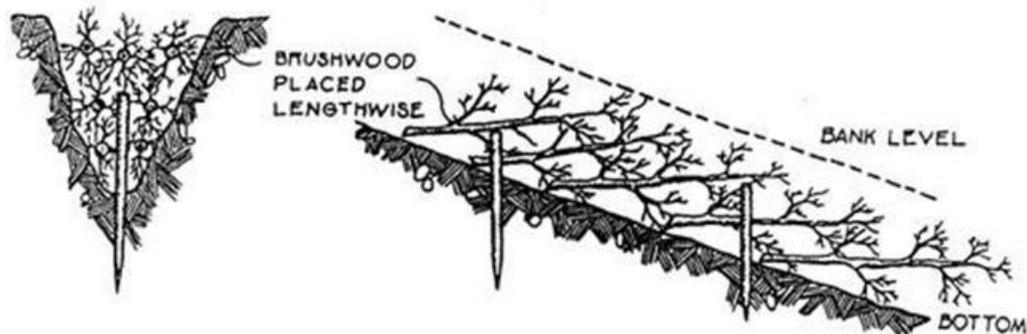
Figure 87. Plugging of small gullies (Source: Manual of Reforestation and Erosion Control, Agpaoa *et al.*,1975).
