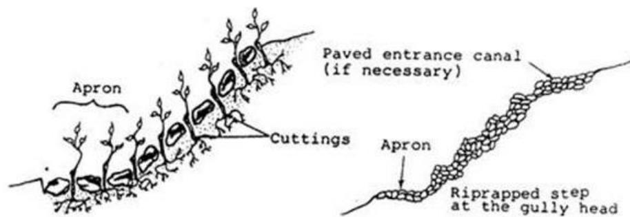
Figure 74. Stabilization of a gully head by riprap (Source: Manual of Reforestation and Erosion Control, Agpaoa et al., 1975)
