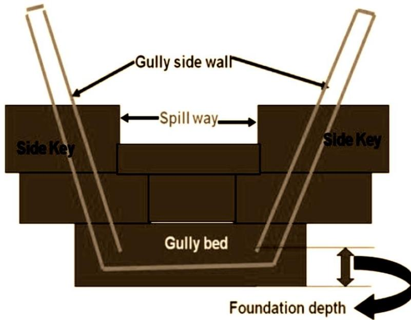
Figure 78. Schematics of gabion and Stone checkdams
