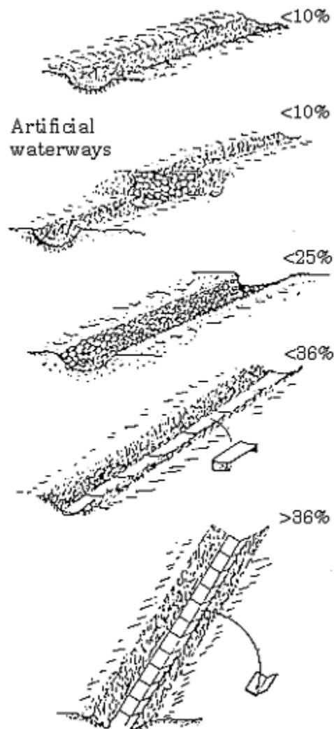
Figure 67. Water ways at different slopes and the required amendments in structure
