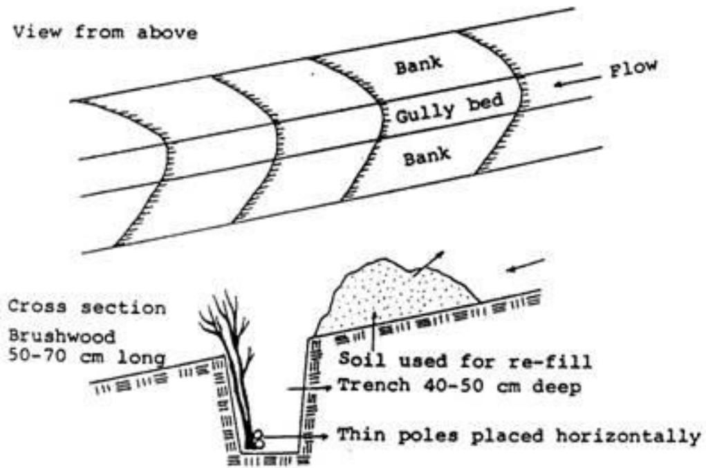
Figure 86. Construction of “brush combs” (Source: Manual of Reforestation and Erosion Control, Agpaoa *et al.*, 1975)
