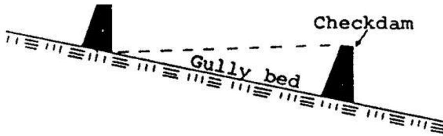
Figure 77. Spacing of checkdams (Source: Manual of Reforestation and Erosion Control, Agpaoa et al.,1975)
