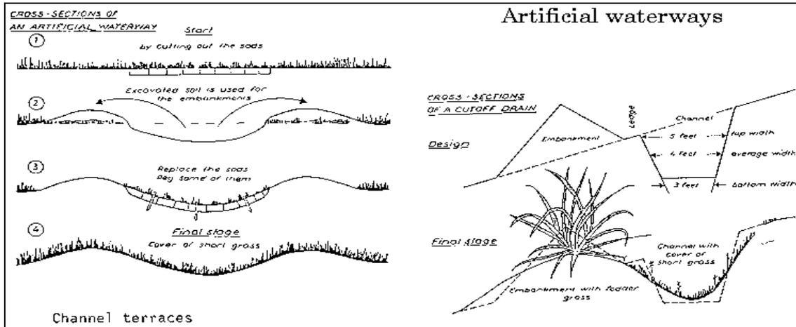
Figure 69. Cross-section of an artificial water way
