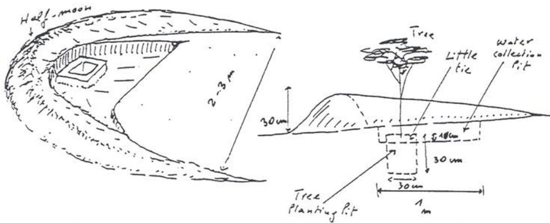
Figure 64. Design and construction of half-moon structure
