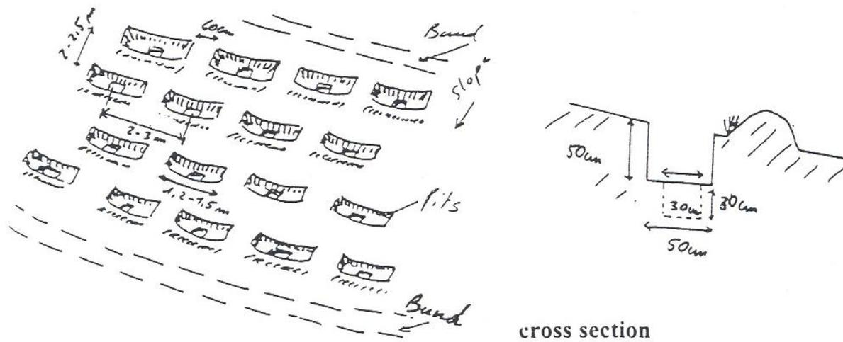
Figure 65. Improved pits along the contour
