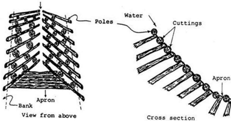
Figure 75. Gully head stabilisation by a pole structure (Source: Manual of Reforestation and Erosion Control, Agpaoa et al., 1975)
