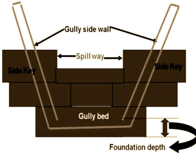
Figure 100. Schematics of gabion and Stone checkdams
