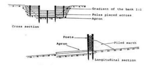
Figure 105. Pole or log checkdam (Source: Manual of Reforestation and Erosion Control, Agpaoa *et al.*,1975)
