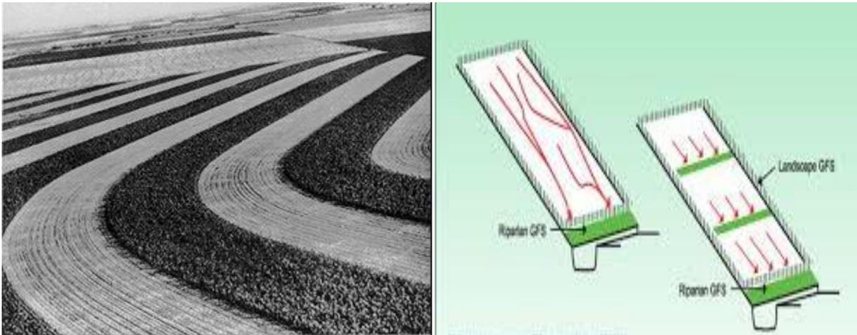
Figure 73. Grass Strips: schematics; and plot with and without grass strip
