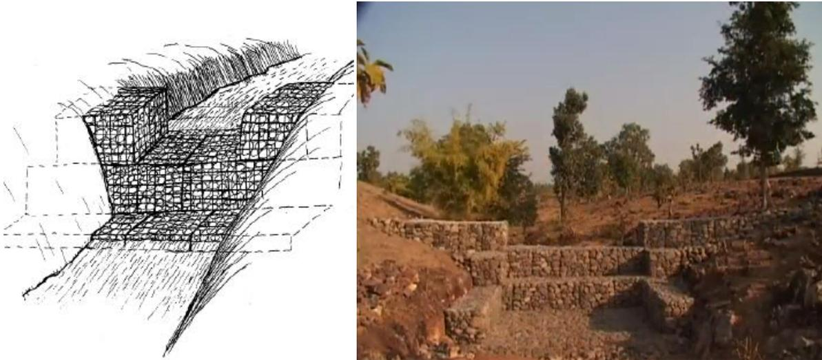
Figure 102. Gabion box checkdams (Source: Manual of Reforestation and Erosion Control, Agpaoa *et al.*, 1975)
