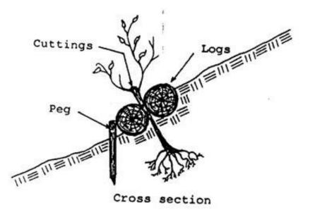
Figure 107. Ground tie with sprouting brushwood (Source: Manual of Reforestation and Erosion Control, Agpaoa *et al.*, 1975)
