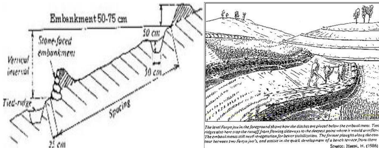
Figure 75. Design of Level Fanya juu, schematics and terminologies
