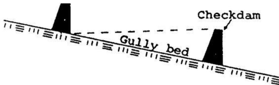
Figure 99. Spacing of checkdams (Source: Manual of Reforestation and Erosion Control, Agpaoa et al., 1975)
