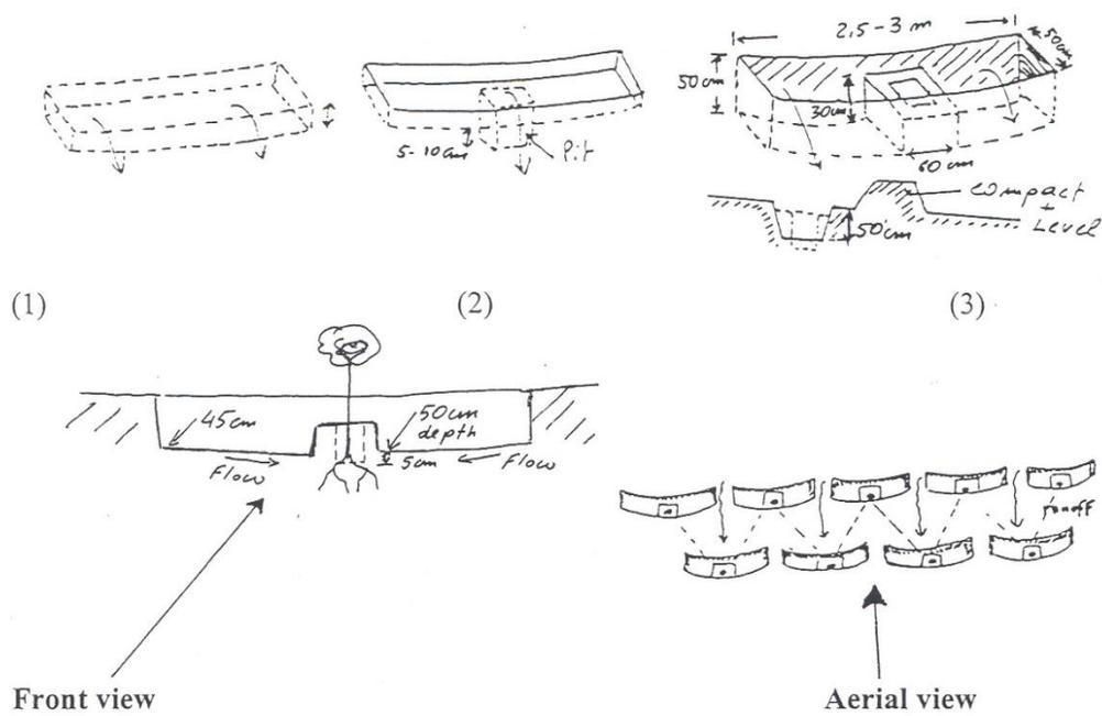
Figure 79. Design of water collection trenches
