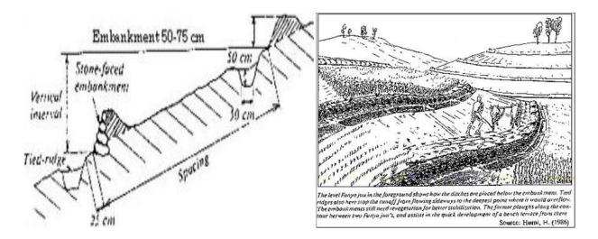
Figure 75. Design of Level Fanya juu, schematics and terminologies
