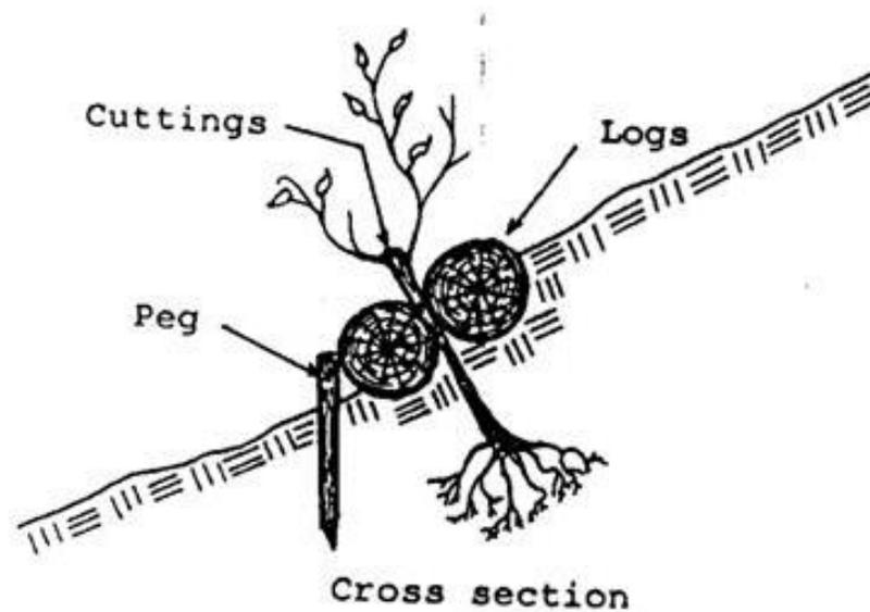
Figure 107. Ground tie with sprouting brushwood (Source: Manual of Reforestation and Erosion Control, Agpaoa *et al.*, 1975)
