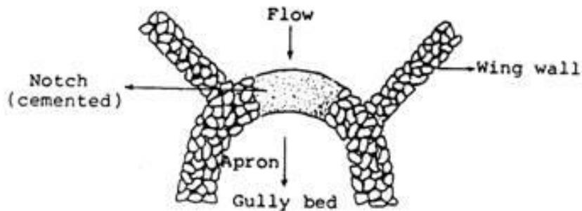
Figure 98. Gully head stabilisation by a solid structure with wing walls (view from above) (Source: Manual of Reforestation and Erosion Control, Agpaoa et al., 1975).
