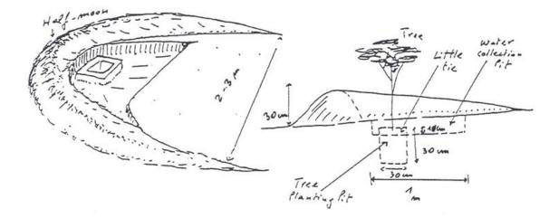
Figure 86. Design and construction of half-moon structure
