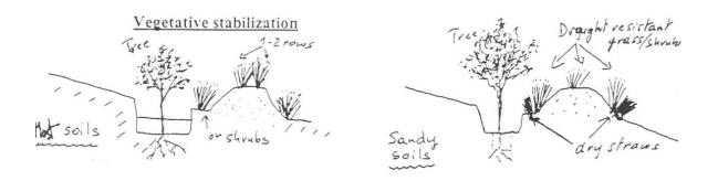
Figure 80. Vegetative stabilization of water collection trenches
