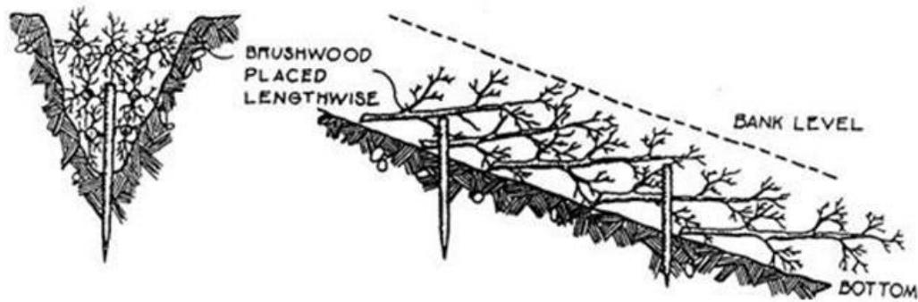
Figure 109. Plugging of small gullies (Source: Manual of Reforestation and Erosion Control, Agpaoa *et al.*,1975).
