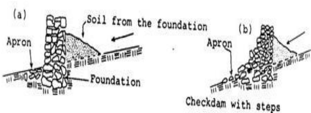
Figure 101. Dry stone checkdams (Source: Manual of Reforestation and Erosion Control, Agpaoa *et al.*, 1975)
