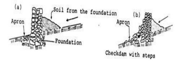
Figure 101. Dry stone checkdams (Source: Manual of Reforestation and Erosion Control, Agpaoa *et al.*, 1975)
