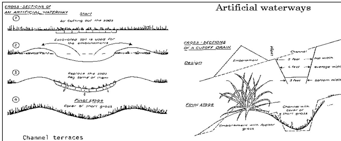
Figure 91. Cross-section of an artificial water way
