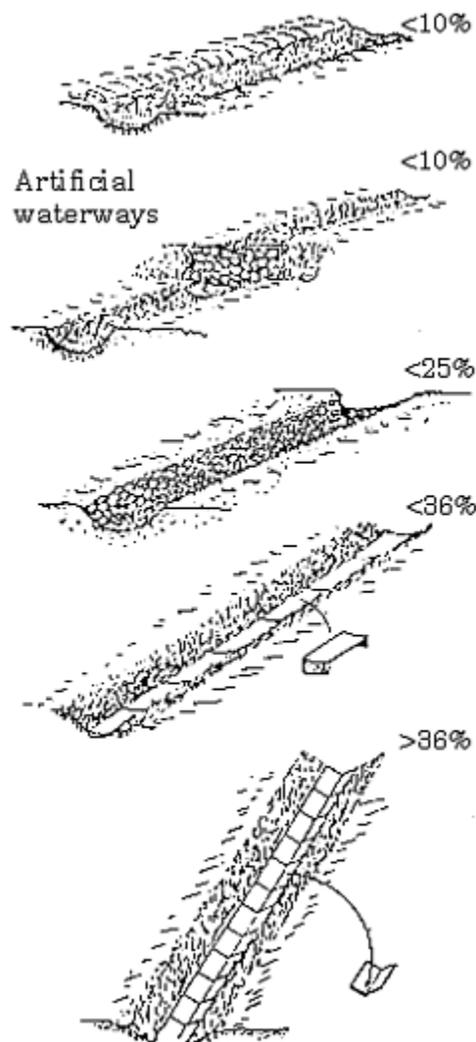
Figure 89. Water ways at different slopes and the required amendments in
