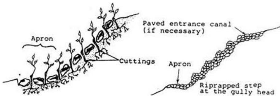
Figure 96. Stabilization of a gully head by riprap (Source: Manual of Reforestation and Erosion Control, Agpaoa et al., 1975)
