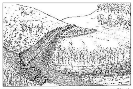
This cutoff drain protects the terraced cultivated land to the right from excessive funoff from the grassiand to the left and above, where controlled grazing is used with tied catile. At the point where the cutoff drain enters the waterway, stone protection is needed and a checkdam has been made in the waterway just below the entry point as shown. Cutoff drains have to be covered with vegetation much more than on the recently constructed embankment shown here.
