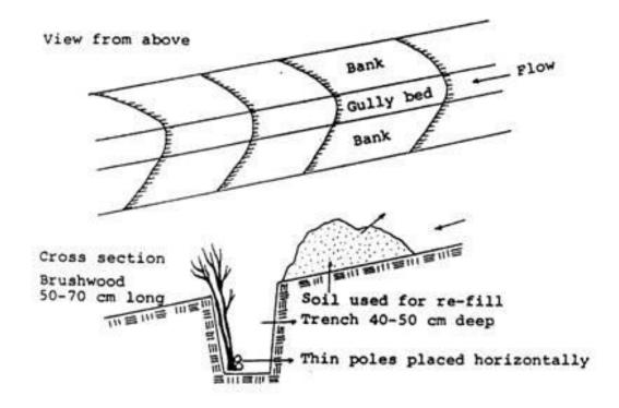
Figure 108. Construction of "brush combs" (Source: Manual of Reforestation and Erosion Control, Agpaoa *et al.*,1975)
