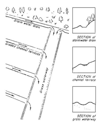
Figure 90. Grass water way and the input system sections
