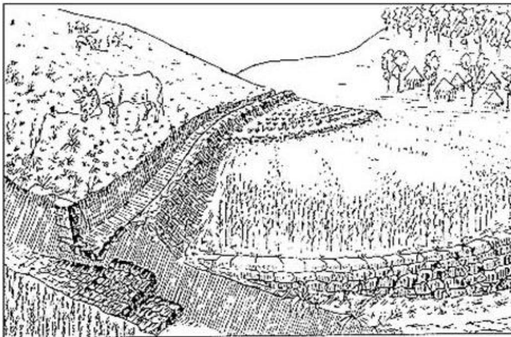
*This cutoff drain protects the terraced cultivated land to the right from excessive runoff from the grassland to the left and above, where controlled grazing is used with tied cattle. At the point where the cutoff drain enters the waterway, stone protection is needed and a checkdam has been made in the waterway just below the entry point as shown. Cutoff drains have to be covered with vegetation much more than on the recently constructed embankment shown here. Source: Hurni, H. (1986)*
