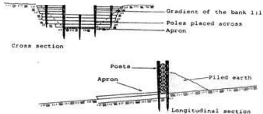
Figure 105. Pole or log checkdam (Source: Manual of Reforestation and Erosion Control, Agpaoa *et al.*, 1975)
