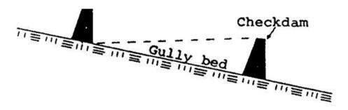
Figure 99. Spacing of checkdams (Source: Manual of Reforestation and Erosion Control, Agpaoa et al.,1975)
