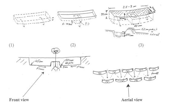
Figure 79. Design of water collection trenches
