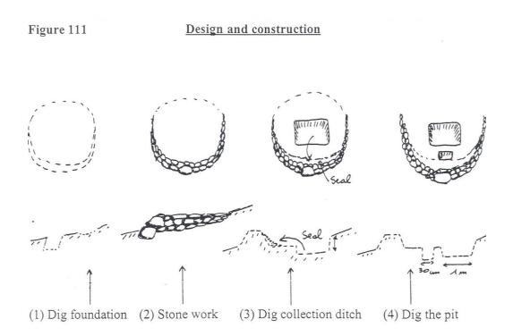
Figure 84. Construction steps of eyebrow basins
