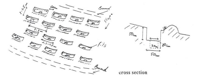
Figure 87. Improved pits along the contour
