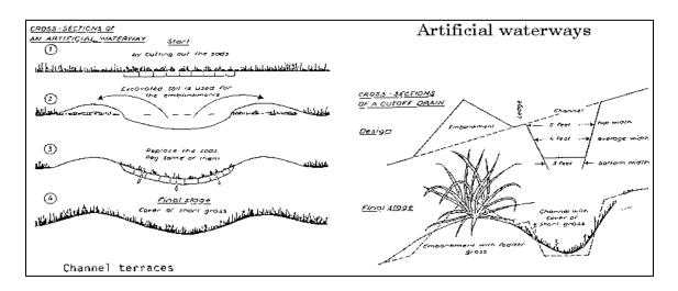
Figure 91. Cross-section of an artificial water way
