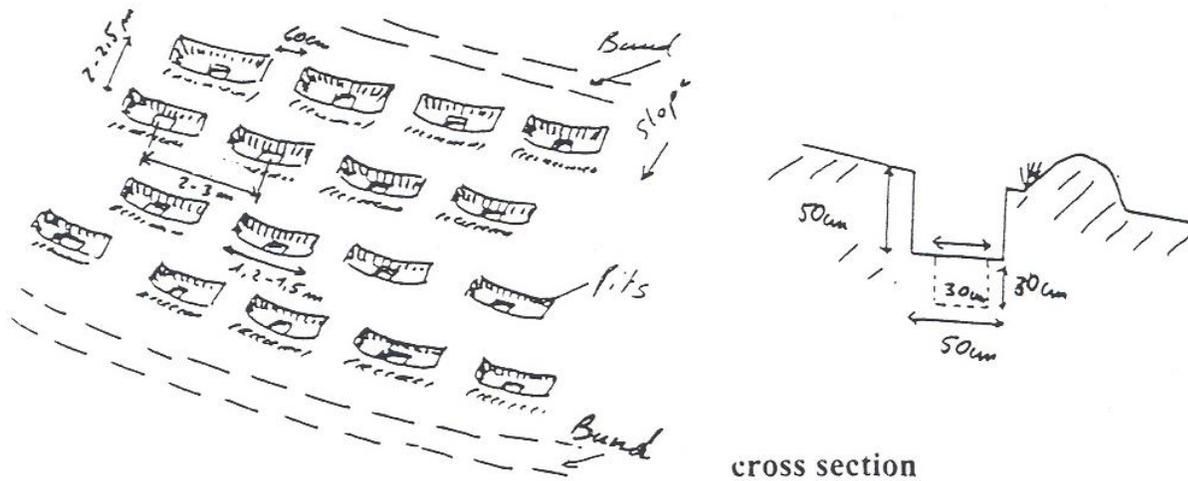
Figure 87. Improved pits along the contour
