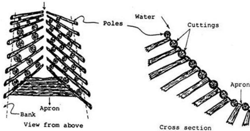
Figure 97. Gully head stabilisation by a pole structure (Source: Manual of Reforestation and Erosion Control, Agpaoa et al., 1975)
