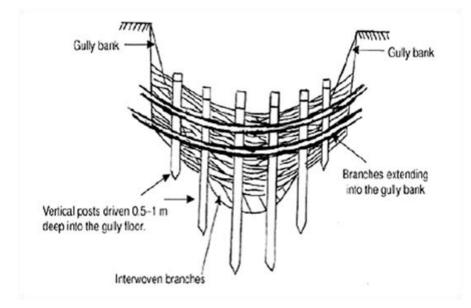
Figure 104. Brushwood checkdams (Source: Manual of Reforestation and Erosion Control, Agpaoa *et al.*, 1975)
