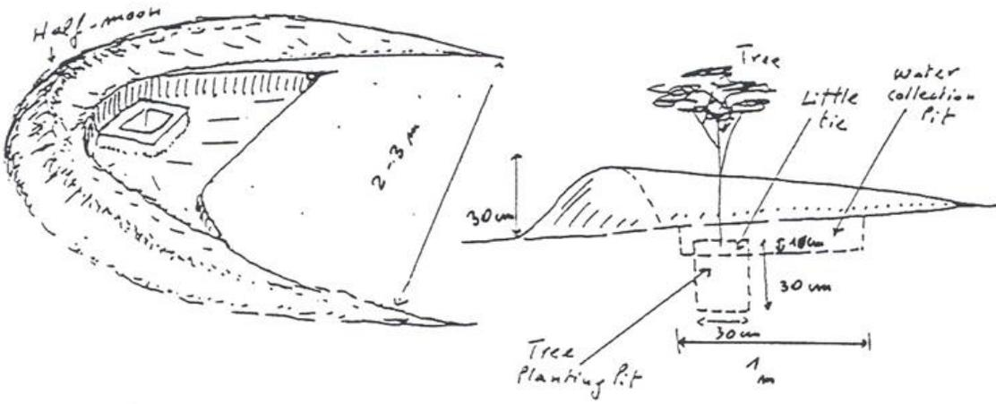
Figure 86. Design and construction of half-moon structure
