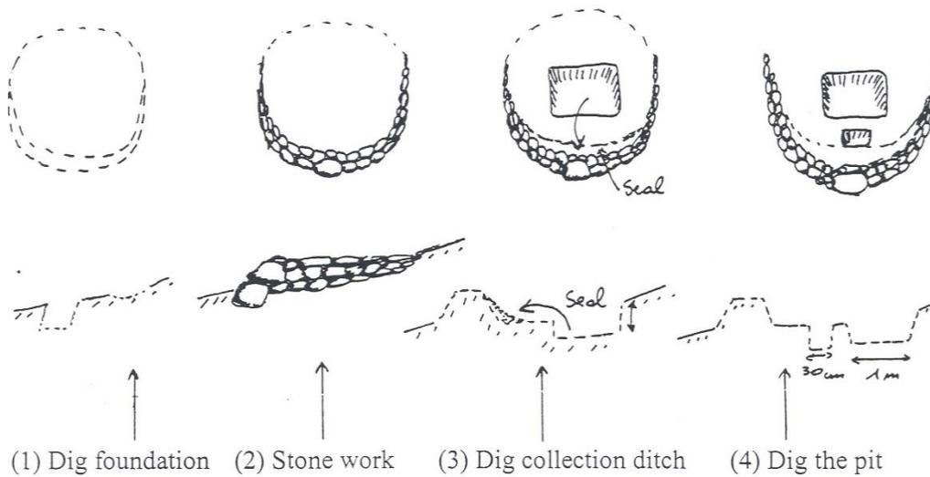
Figure 84. Construction steps of eyebrow basins
