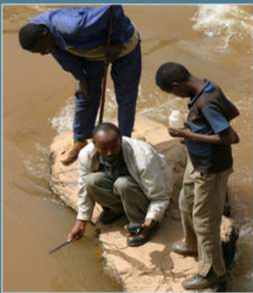
Mr. Demise Alamirew, a hydrologist (middle), working with his team on sampling and measurement of temperature, acidity and conductivity of the surface water at the Birbir River near Yubdo town.
